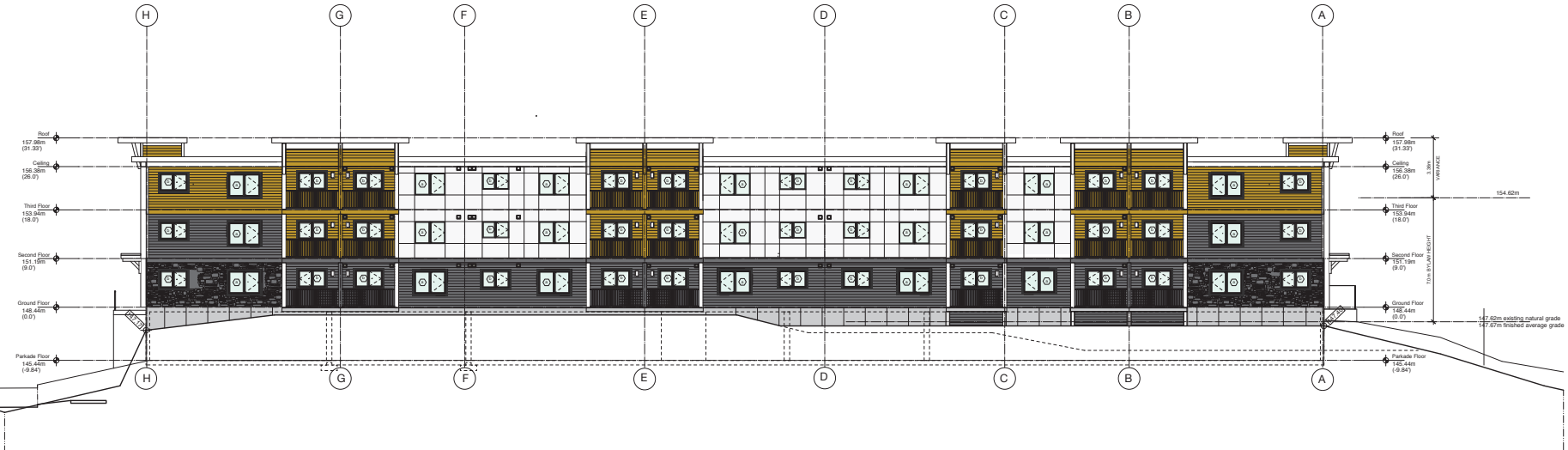
1 Building C - Southeast Elevation 1/8"=1'-0"
